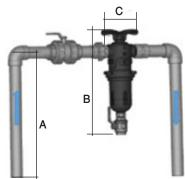
We recommend installing a manual valve in the upstream.
