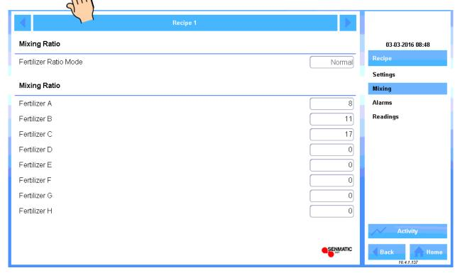
Set the needed mixing ratio between your stock solution tanks, containing the different types of fertilizer. The numbers in this example, 8, 11 and 17 means that 8+11+17=36=>100%
