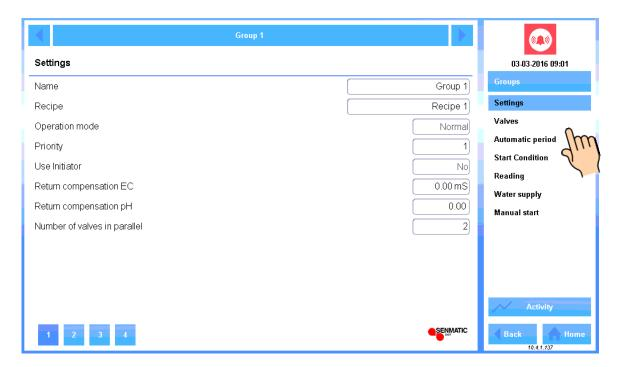
Be sure that the correct Recipe is selected. Number of valves in parallel is normally 1, but 2 or more can be opened at the same time if the capacity is sufficient. "Group 1" can be renamed. Maybe "West" is a better name.
