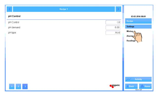
Turn on pH control if needed and set the desired pH demand. Acid is normally used for pH control, but if you use alkaline, you must change pH type.
